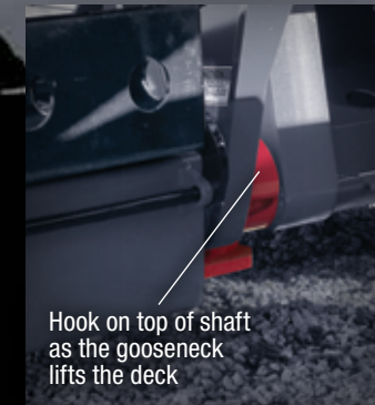
3. When the gooseneck contacts the deck you are in position to lift the trailer
