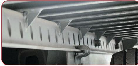
Welded steel reinforcing gussets increase torsional stiffness and strength for superior slider rail stability.
