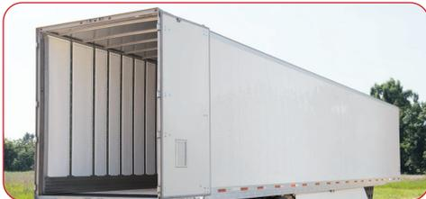
Corrosion resistant frame reduces maintenance costs and increases resale value. The 110½" door opening height allows increased forklift clearance.
