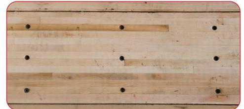
The high payload floor system is standard with a 20,000 lb fork truck front axle floor rating and three screws per floor board.
