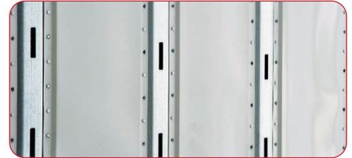
Engineered and track tested to create optimal side wall strength, the design also provides 101" of inside width, and greater cargo securement versatility.
