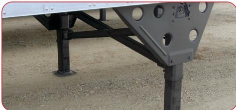
Formed channel cross braces and high strength steel aerospace-style wingplates maximize strength and reduce tare weight. 5-year maintenance-free lubrication package included.
