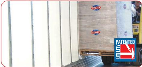
Galvanized interior lining is squeeze riveted with fully recessed fasteners to outer skin and side posts, creating a **Snag-Free®**, high strength composite wall.
