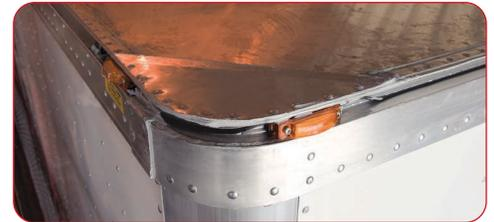
Our bi-directionally tensioned aluminum roof skin has diagonal reinforcing plates at all four corners. It is supported by anti-snag roof bows and is mechanically crimped around the top rail for moisture entry protection.
