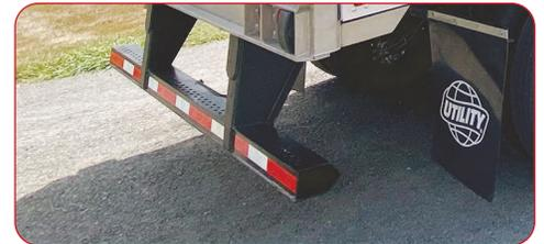
Fully integrated into the rear threshold assembly, this high strength steel bumper complies with U.S. D.O.T. and Transport Canada safety regulations. The 7" deep horizontal bumper provides superior strength and protection.
