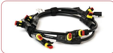
The sealed main harness features 100% soldered internal connectors to prevent corrosive de-icing chemicals from traveling through connections into the wiring.
