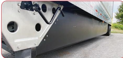
SAE tested and SmartWay®-verified to improve fuel savings, the Utility Side Skirt is also CARB-compliant when used with low rolling resistance tires.
