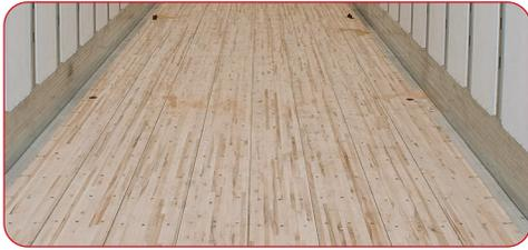
Flooring is pre-undercoated to extend floor life. Weatherproof sealant is applied between every floorboard. Utility-designed gaskets are installed between the troughs and bottom rails for leak protection.
