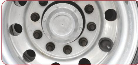
ConMet PreSet Plus includes iron hub, seals, bearings, spacer and spindle nut. This premium system also comes with an 8-year warranty.
