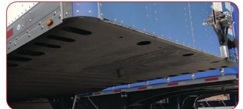
Approach plate is supported by six formed "toes-down" channels to prevent dishing. The kingpin is AAR-rated and the whole assembly is secured to the bottom rails with stainless steel rivets.
