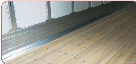
Low-profile 80,000 psi high-strength galvanized steel wearband provides added impact protection, strength, and stiffness.
