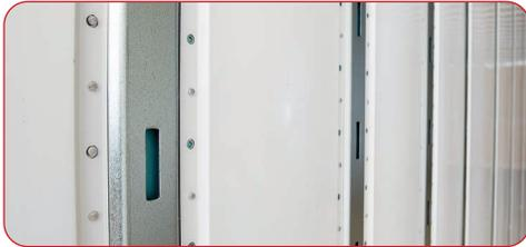
Securely bonds exterior skin with interior lining panels for remarkable side wall strength, increased durability, and reduced tare weight.
