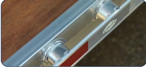
Additional pipe spools can be added to provide increased load protection.
