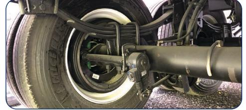
Spring suspension is a light weight option to increase payload, reduce maintenance and lower overall costs.
