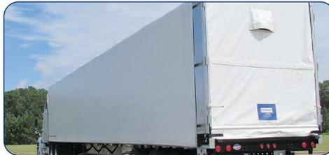
Simple to operate, Conestoga XP offered by Utility is a sliding tarp system that protects loads from the elements without costly and time-consuming tarping.
