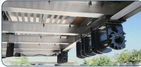
Integrated into the extruded aluminum side rails on both sides of the flatbed, sliding winches are designed to increase load securement versatility.
