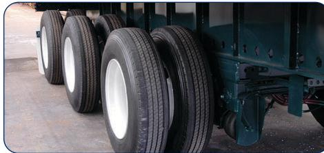
Tri-axle suspension options with 49", 60" and 72" spread axles provide higher payload capacity.
