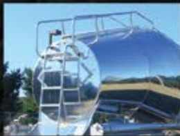
Transition Walkway with Handrails
