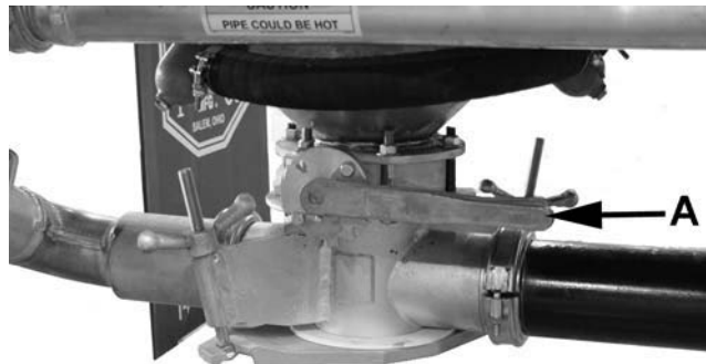
Figure 5-1 – Discharge Valve Closed
