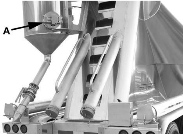
Figure 7-1 – Filter Tank Door
