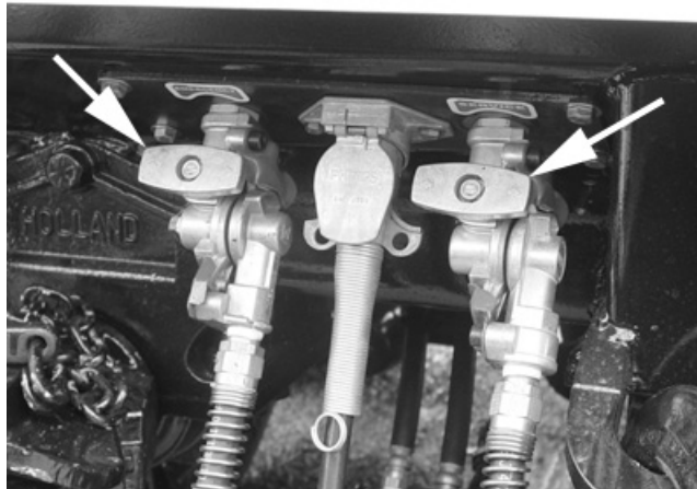
Figure 6-1 Air Supply Valves On Lead Trailer
