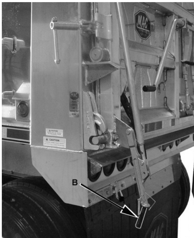
Figure 5-5 Pull Down On Ground Control Handle
