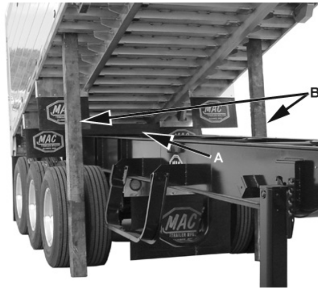
Figure 8-1 Block Up Dump Body
