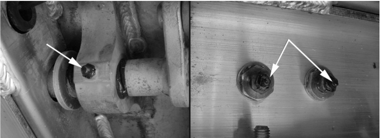
Figure 8-7 Tailgate Latch Bar Bearing and Remote Grease Fittings
