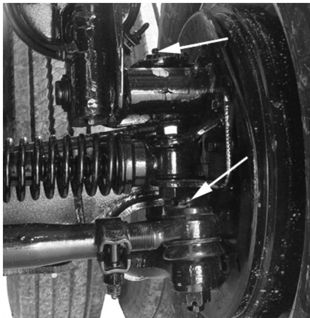
Figure 8-8 Steerable Axle Grease Fittings
