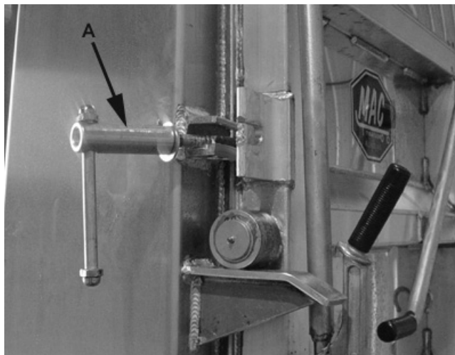
Figure 5-2 Open Winder On Tailgate
