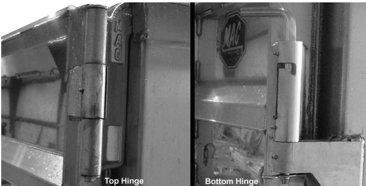
Figure 5-3 Side Swing Hinges Properly Engaged
